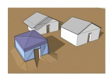
t COVER BAG WALLS. Use earth plaster under roof overhangs or in dry climates. On exposed walls use a protective topcoat, embed tile or pebbles in earth plaster, or use cement plaster on sandy earthbag fill. Mesh, like fishnet, will strengthen both walls and plaster. Cover temporary walls with tarps to last more than 1 or 2 months in full sun.
